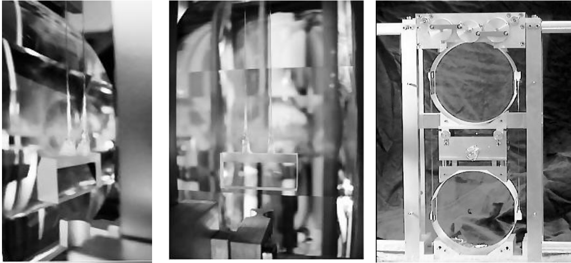
Figure 2. Side view (left panel) and oblique view (centre panel) of a GEO 600 mirror, showing the attachment of fused-silica fibres. A fused silica ear is bonded to the substrate and the fibres are subsequently welded to the ear using an oxy-hydrogen flame. The welding is done in a jig (right panel) which is then used to support the suspension as it is installed in the vacuum tank and hung from the top suspension mass on a pair of loops of steel wire which pass round the upper of the two masses shown.
