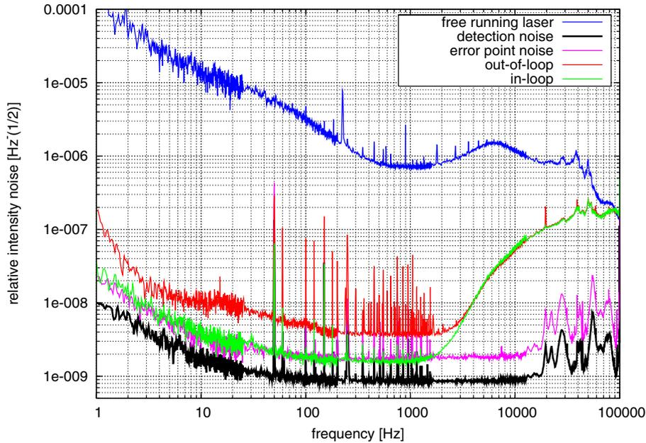
**Figure 3.** Relative power noise of a free-running and stabilized 12 W laser system. The gain in the control loop is sufficient to bring the in-loop result close to the AdvLIGO requirements. The discrepancy between the in-loop and the out-of-loop result is not understood and subject of ongoing investigations.
