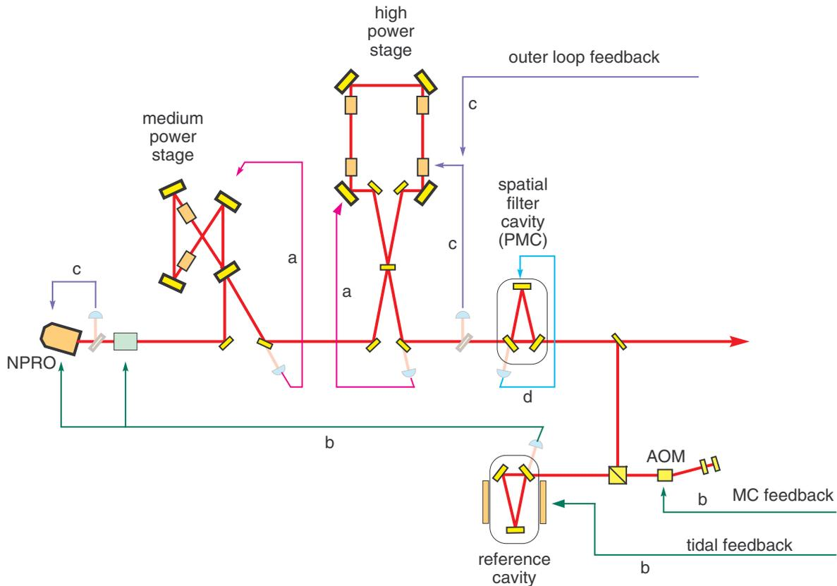
**Figure 2.** Stabilization scheme of the Advanced LIGO PSL . The different control loops are ordered by function. a: injection locking, b: frequency stabilization, c: power stabilization, d: length control of the filter cavity
