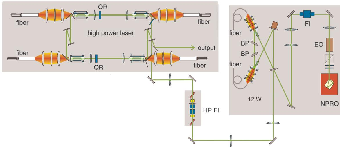
**Figure 1.** Optical layout of the 200 W laser: The beam from a 12 W injection-locked laser system is injected into the high-power slave-cavity which uses two pairs of birefringence compensated end-pumped Nd:YAG rods. The 12 W stage is injection locked to an 800 mW NPRO that provides a high frequency stability that is inherited by both injection locking stages. FI: Faraday Isolator, EO: electro-optical modulator, HPFI: high power Faraday Isolator, BP: Brewster plate, QR: quartz rotator
